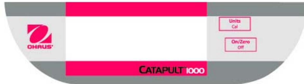
Unit/Cal – Short press scrolls through active units and modes (kg, kg dynamic)
